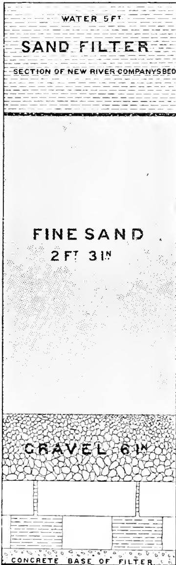
Diagram of a section of a sand filter.
